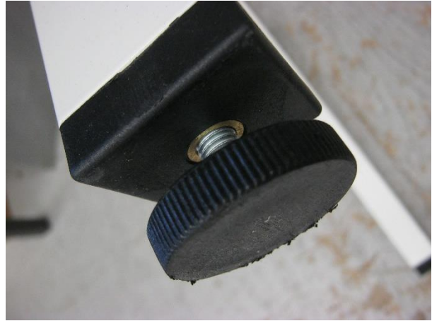
Photo 6: Tested sample 220609-3 of Techo Fount Classic A-Leg - detail final leveller
