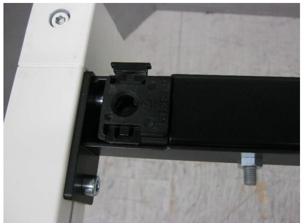
Photo 4: Tested sample 220609-3 of Techo Fount Classic A-Leg - detail connection legs to frame
