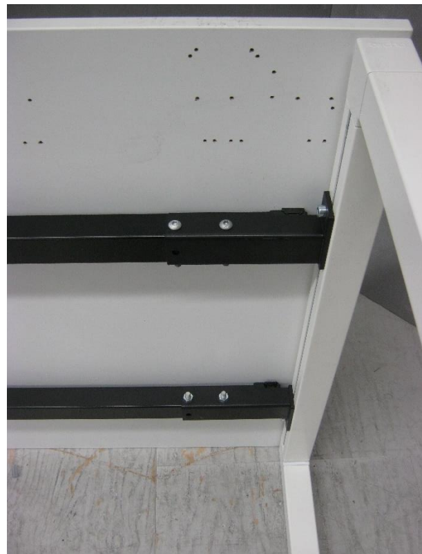
Photo 4: Tested sample 220609-2 of Techo Fount Classic N-Leg office desk - detail connection legs to frame
